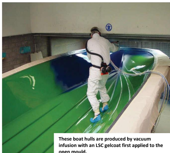
**These boat hulls are produced by vacuum infusion with an LSC gelcoat first applied to the open mould.**
