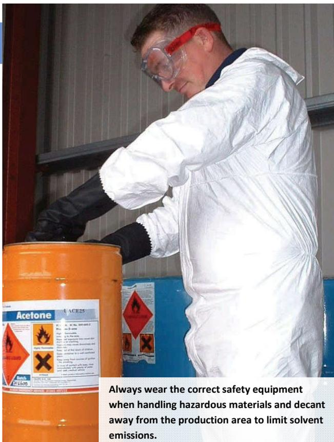
Always wear the correct safety equipment when handling hazardous materials and decant away from the production area to limit solvent emissions.
