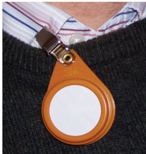
Badge monitoring and data analysis system for recording workplace styrene
